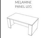
Melamine panel leg, thickness 38mm, ABS edge banding thickness 2 mm adapted to the finish. Consists of a panel the depth of the worktop with an L. 200 mm return to the front face. Structural Aluminium grey metal crossbeam, cross-section 60 x 30 mm, thickness 2 mm Melamine modesty board H 300 mmm thickness 19 mm
