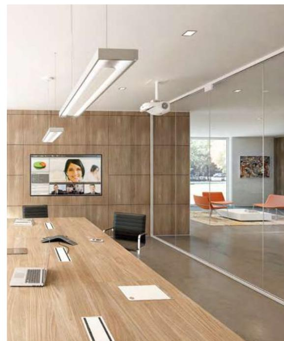
Collectivity and privacy, transparency and transformation with electrochromic glass. The crystalline transparency of the wall panel can vary. Constant visual contact with the surroundings can change, by customising the space and separating the setting from its context by switching the smart electrochromic glass, which turns the transparent surface matt to create privacy for a meeting or to project onto the glazed surfaces.
